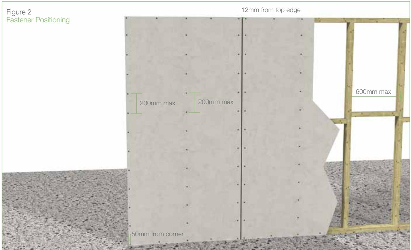
Durascpae™ panels should be installed vertically with all sheet edges fully supported. The centre joints must coincide with the
