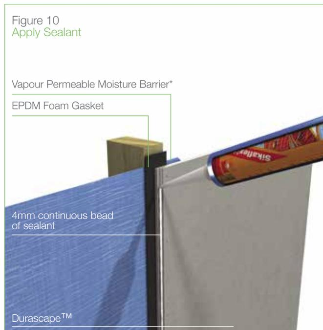
Once both sheets are fixed, check the joint for gaps and fill with additional sealant if required.
