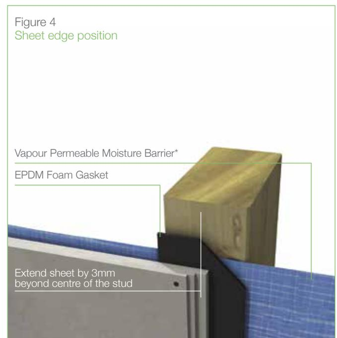
Position the underlap sheet on every stud 3mm past the centre of the stud to ensure the fasteners fixed at the edge of the sheet have adequate distance into the stud.
