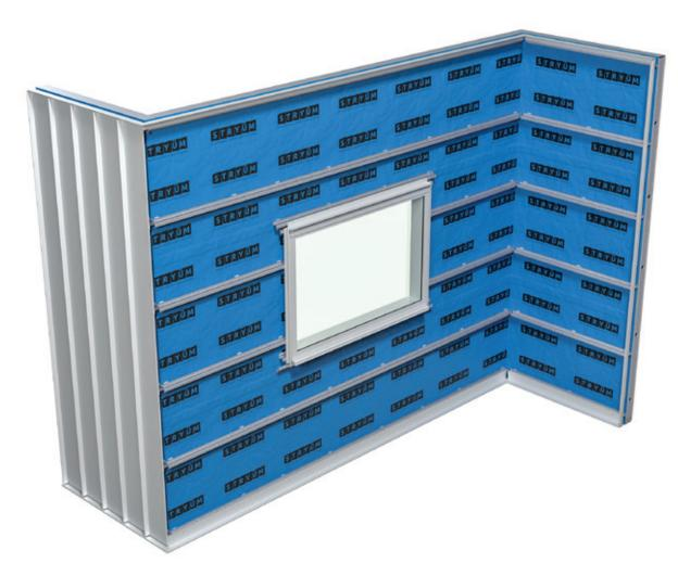
Install the cladding by cutting the panels to length, hooking the panel into the previous panel, and affixing to the S Batten. In this diagram the cladding direction chosen is Left-Right. Due to the rainscreen façade system Stryüm utilizes, a minimum airflow gap of 10mm must be maintained at the top and bottom of the cavity.
