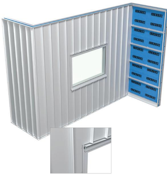
Install the cladding by cutting the panels to length, hooking into the previous panel, and affixing to the S Batten.
