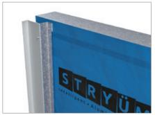
Install the vertical trims for the cladding, at the left and right of the cladding section, at either side of any wall penetrations, and at any corners. When installing down to an adjacent flat surface such as a garden bed or pathway, a minimum of 150mm from the ground is recommended to prevent rain splash back dirtying the façade.
