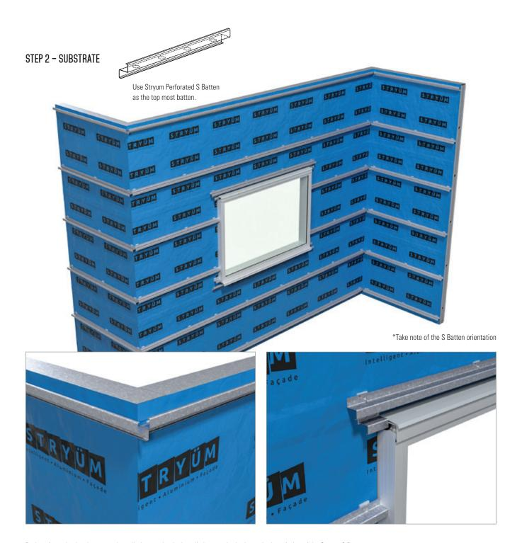
Packers for a plumb substrate and ventilation need to be installed as required prior to the installation of the Stryüm S Batten.
