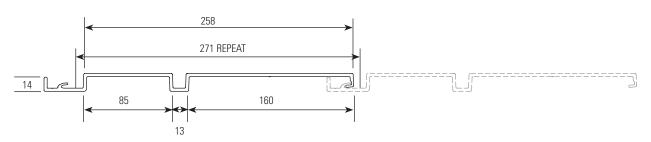
Thickness: 3mm Weight: 10.94kg/m² Length: 6.5m Effective Cover: 271.1mm per panel
