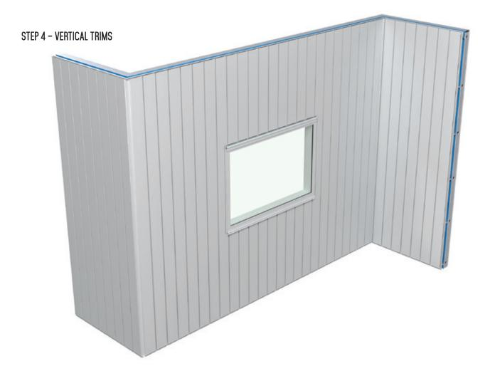
Install the cladding by cutting the panels to length, hooking the panel into the previous panel, and affixing to the S Batten. In this diagram the cladding direction chosen is Left-Right.
