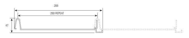
Thickness: 2.8mm Weight: 11.07kg/m² Length: 6.5m Effective Cover: 260mm per panel
