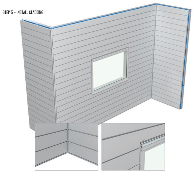
Install the cladding by cutting the panels to length, hooking the panel into the previous panel, and affixing to the S Batten. Due to the rainscreen façade system Stryüm utilizes, a minimum airflow gap of 10mm must be maintained at the top and bottom of the cavity.
