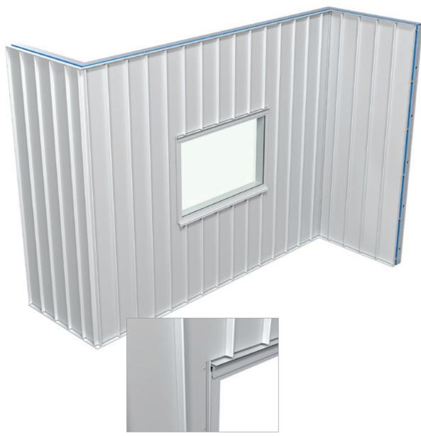
Install packers adjacent to TRM0201b and trim the raised hook/starter section from the length of the Seam panel. Install this trimmed first panel up against TRM0201b and fix through the face of the cladding into the packers.
