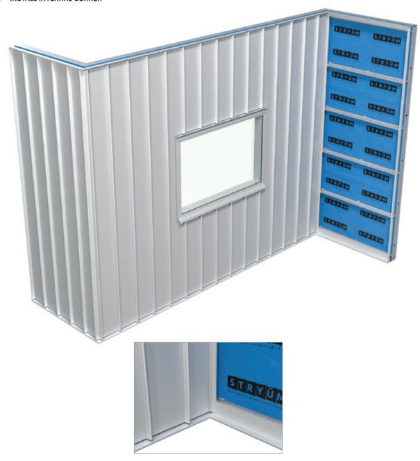
Install TRM0201b Female into the internal corner.
