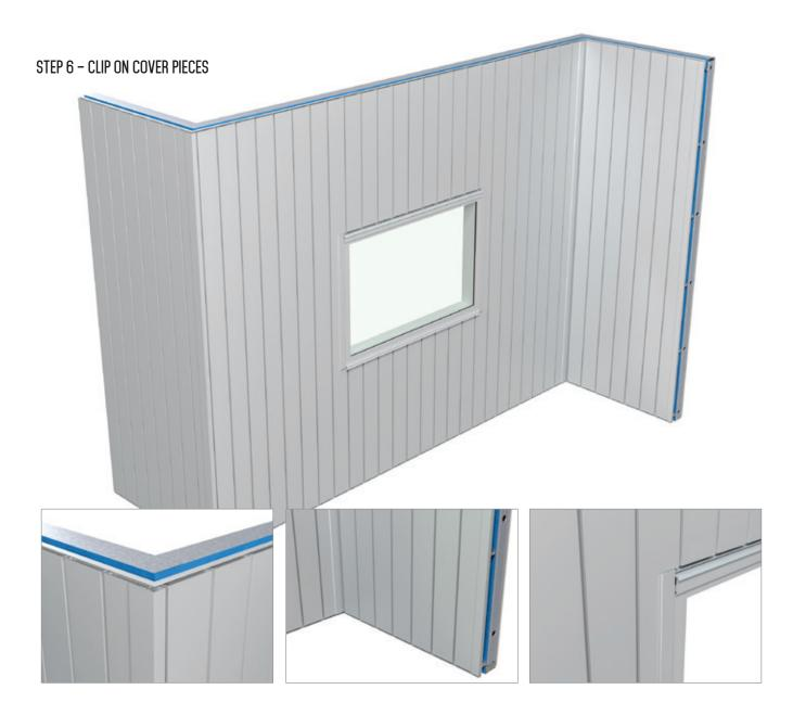
Install the cover sections to the two-piece trims to conceal rivets and cut edges. Push firmly into place, a rubber mallet may be used paying careful attention to the finish.
