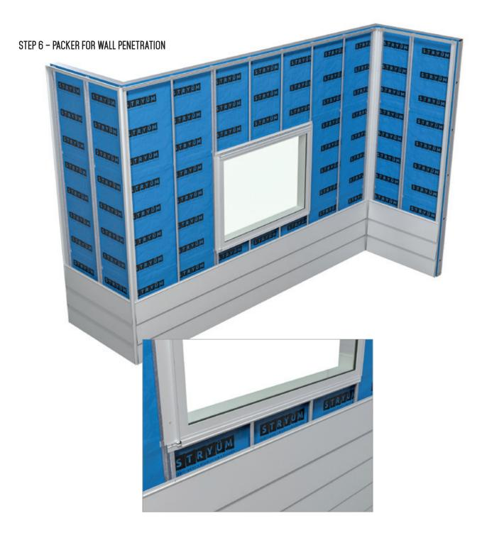
Due to the sloping nature of Step, the depth packer required to support the panel around wall penetrations will depend on where the penetrations sit down the panel. Measure carefully where the panel needs to be cut, and calculate the packer required before.
