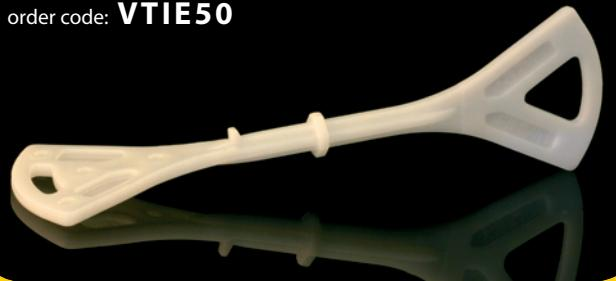
50mm side fixed Veneer Ties in Medium duty (white) to satisfy AS/NZ 2699-2000. Use 2 fixings to prevent rotation whilst in service. Colour coded to assist in identifying classification in the wall. Ideal for steel and timber stud, brick veneer homes and buildings.
