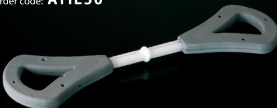
50mm Acoustic Cavity tie is the standard medium duty Ni-Tie with each end over moulded with a resilient material. The resilience substantially reduces air and structure borne noises. Also reduces impact and vibration in masonry walls.
