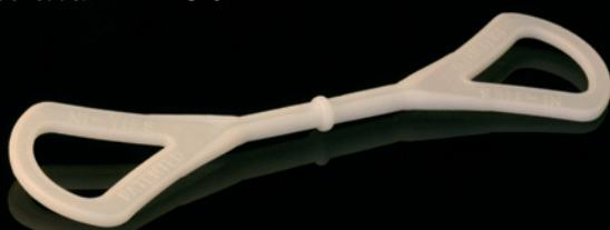
50mm Cavity Ties in Medium duty (white) to satisfy AS/NZ 2699-2000. Rounded ends to prevent injury and central hole to assist bond in mortar.
